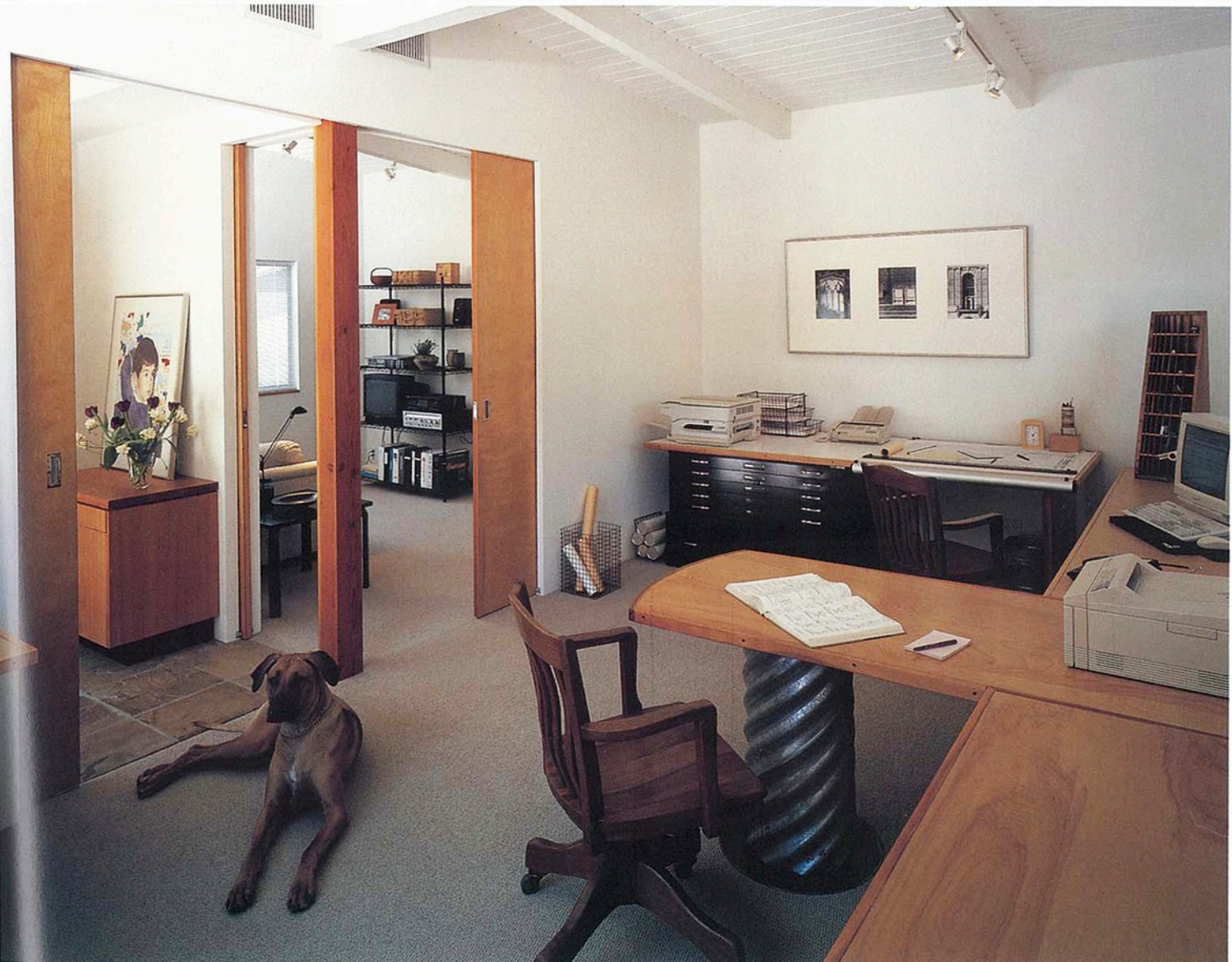
▲The arrangement of pocket doors around a center post allows for a variety of space configurations to accommodate changing work situations, visitors, and guests.
